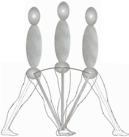
Fig. 1. - During each walking step, the center of body mass vaults over the supporting limb like an inverted pendulum.
